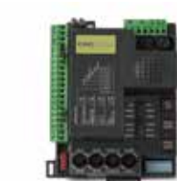
STARG824NG - COD. 12S021 Control unit for 24 Vdc motors (without transformer and external box)
